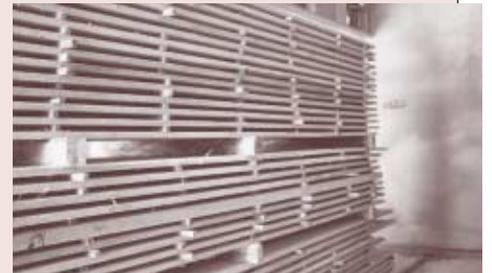
**ABOVE:** *After careful sawing and extended air-drying, your wood is slowly dried in our dehumidification kiln to ensure that the wood can be easily acclimated to the site conditions in your home or office.*
