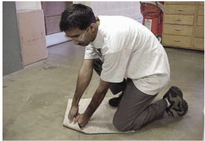
Figure 6-3. The Mat Bond Test is a short-term test installation that does not reveal moisture conditions deep within the floor slab. (IMG15991)
