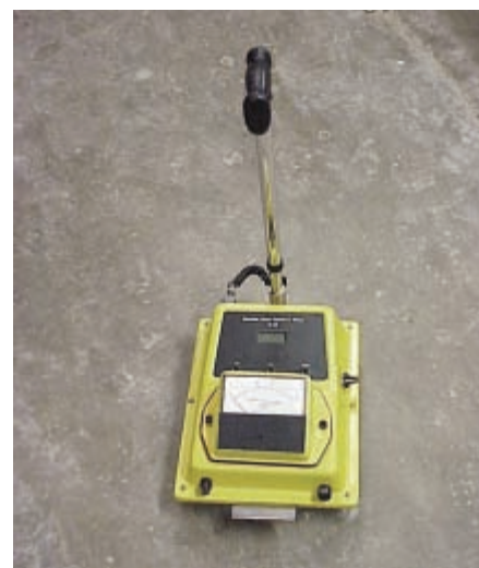
Figure 6-7. Requirements of nuclear moisture gauges for training, licensing, handling, and transport make them less desirable for routine floor testing. (IMG12233)
