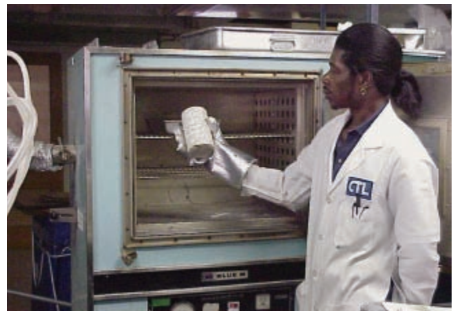
Figure 6-8. Gravimetric moisture analysis determines weight percent of free moisture by heating a concrete specimen to constant weight. Wet-cored cylinders obtained from in-place floors cannot be used for this purpose. (IMG15990)
