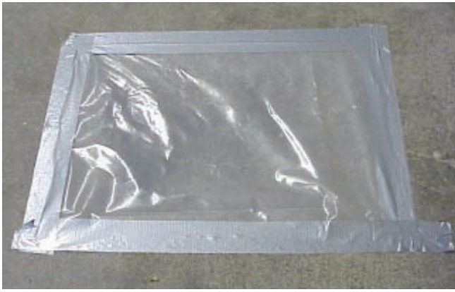
Figure 6-2. False negative results from the Plastic Sheet Test can indicate a floor is dry simply because the concrete surface temperature is above the dew point conditions within the slab. (IMG15992)
