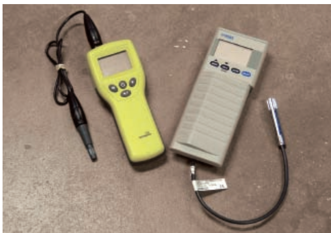
Figure 6-11. RH Probes containing moisture sensors directly determine relative humidity in holes drilled into concrete floor slabs. (IMG15962)
