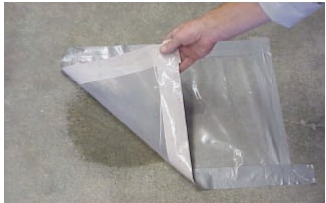
Figure 6-1. Plastic sheet test, ASTM D4263, can show positive results when excessive moisture is present in a concrete floor slab. (IMG15993)
