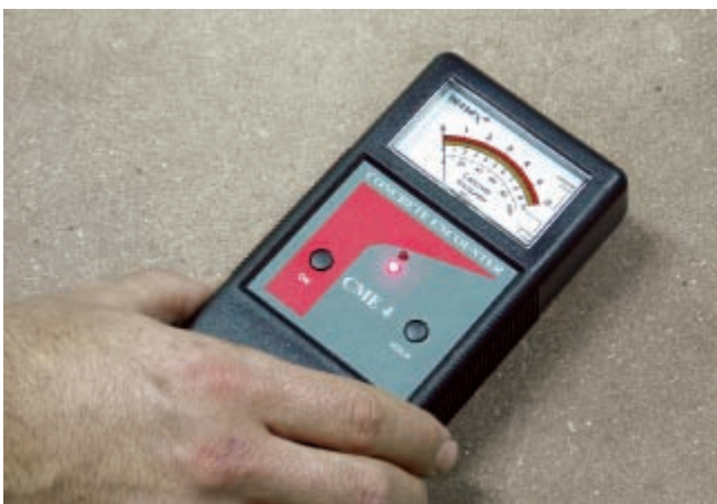
Figure 6-5. Electrical impedance devices can provide comparative measures of moisture in the upper region of a slab. (IMG15963)
