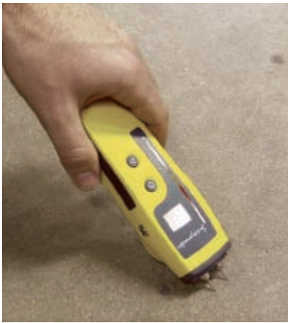
Figure 6-4. Electrical resistance testing may not relate to the true condition of available moisture within a concrete slab. (IMG15964)
