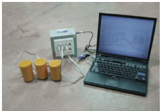
Figure 6-12. RH Probes can be connected to data loggers to record trends in floor moisture and predict when a floor will be dry enough for installation of finish flooring systems. (IMG15961)
