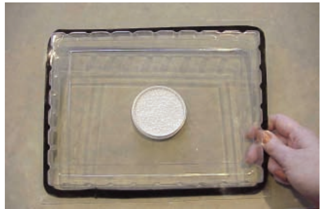
Figure 6-9. Moisture vapor emission rate is determined according to ASTM F1869 using commercially available calcium chloride kits that absorb moisture from a specific test area over a known length of time. (IMG15989)
