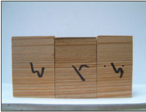
The center piece demonstrates compression set: It was cut, soaked while restrained from swelling, and redried. It is now slightly narrower.
